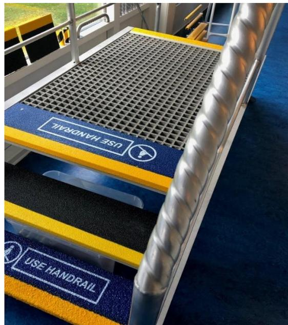
Figure 17: Formed KAG handrail sample. Source: (Appendix 1: Electronic Interviews).
