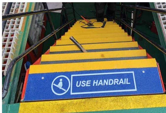
Figure 16: Real Safety anti-slip stair tread covers at Danish ship. Source: Author
