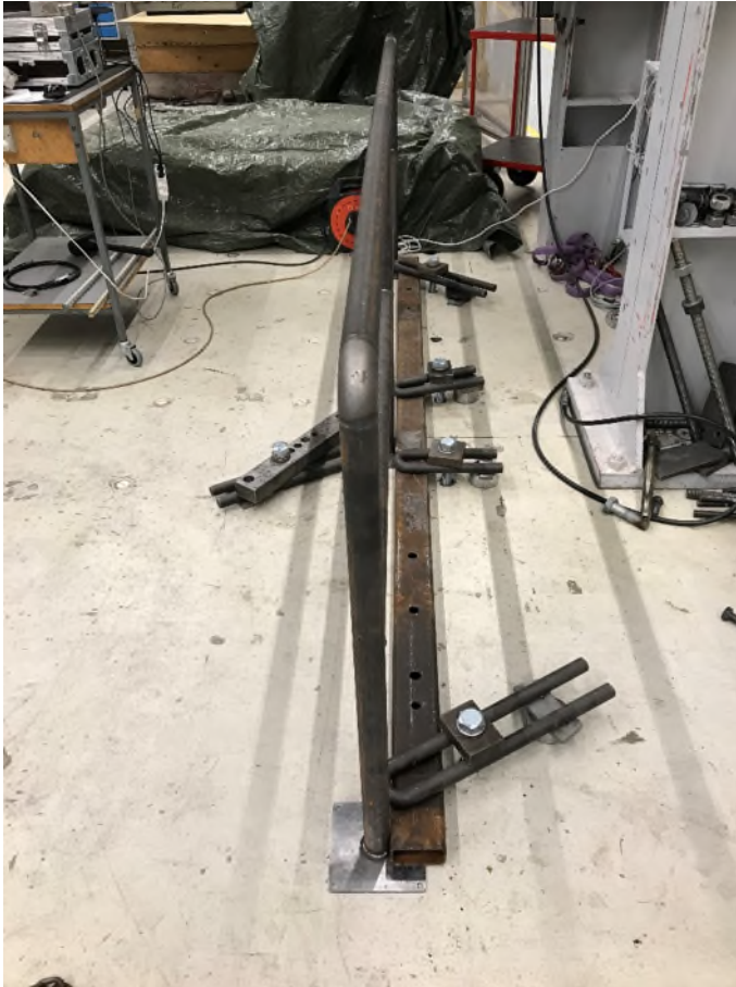
Figure 5 - Guard rail fastening, with an RHS 100x50x4,5mm laid on top of the foot plates.
